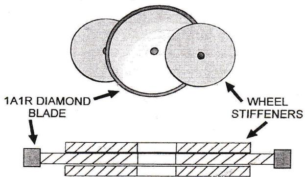
WHEEL STIFFENER SETS Provide Stability to Thin Diamond Blades which helps prevent the blade from "walking". Stiffeners should be used at 2/3rd's the Outside Diameter of the Diamond Blade.
