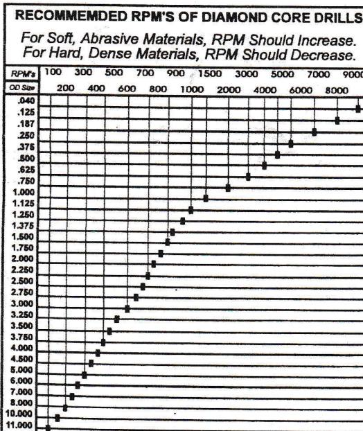
RPM's will vary depending on the OD size of the drill. To improve drill life and help reduce breakage, it is important to run drills at the proper RPM's and keep the diamonds exposed through frequent dressing.
