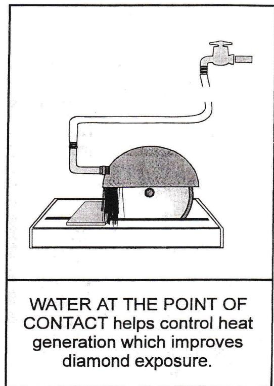
**WATER AT THE POINT OF CONTACT** helps control heat generation which improves diamond exposure.
